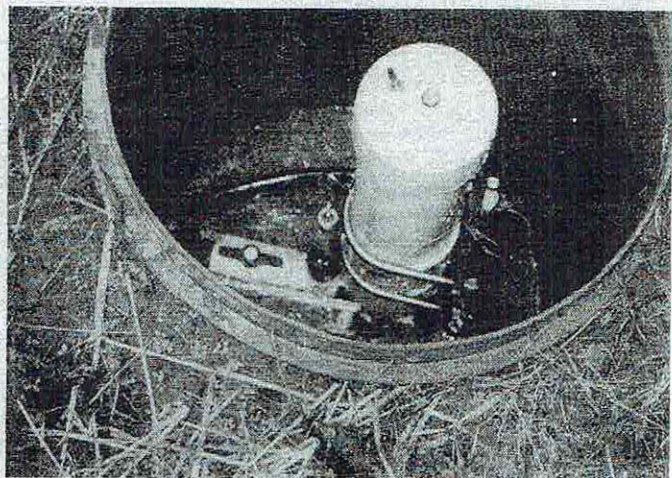
Home-made ram pump submerged in a plastic barrel.
